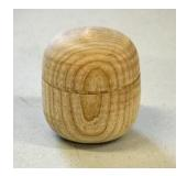
Mark stressed that, for boxes, the wood should be very dry or else the movement that would occur would possibly lock the lid on.
