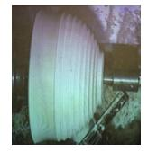
The bowl was reversed in the chuck and Mark cored the centre out for use as the lid. With the core removed the inside was tidied up with a ridge left to support the lid. The inside of the walls of the bowl were undercut slightly and curving nicely to the base of the bowl. He explained that the curving undercut is important so that it is easier to remove any contents that may be placed in the bowl.
